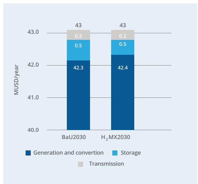
For the **H<sub>2</sub>MX2030** scenario, the electricity storage needs were reduced to 22 GWh, but additional 11 GWh<sub>2</sub> (330 tons of H<sub>2</sub>) were needed in H<sub>2</sub> vessels. Approximately 25% more energy storage was possible in the **H<sub>2</sub>MX2030** scenario compared with the **BaU2030** one at the same cost.
