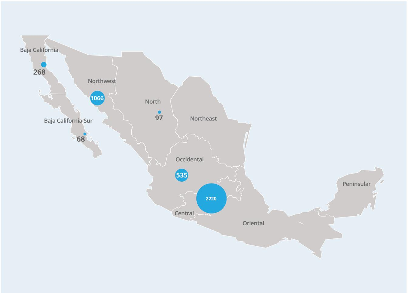
Figure 4-19. shows the distribution of CCGT-H<sub>2</sub> installed capacity by region. In total 1.5 GW of CCGT-H<sub>2</sub> would be needed. The PEMEL and CCGT-H<sub>2</sub> distribution are proportional. There are approximately 3 times more PEMEL installed capacity than CCGT-H<sub>2</sub>.
