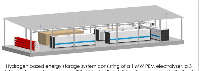
Hydrogen based energy storage system consisting of a 1 MW PEM electrolyzer, a 3 MWh hydrogen storage and a 300 kW fuel cell, stabilizing the power grid in Thailand (for EGAT) with high penetration of wind energy (source: Hydrogenics)
