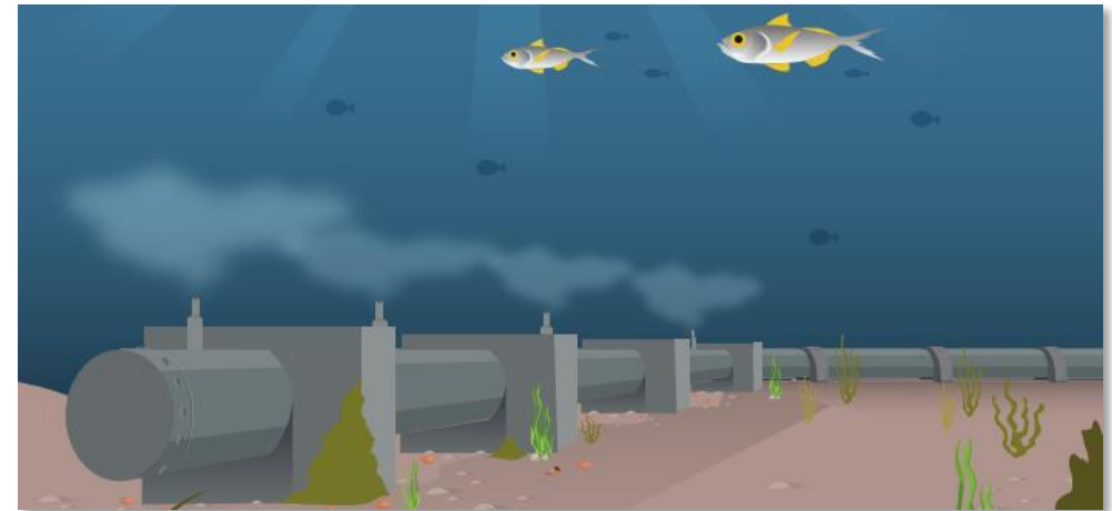
Disposal of brine through multiple diffusers
